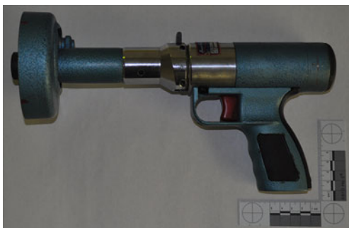
Fig. 4 Carl Bauer “Record Piccolo S”; projectile diameter, d=6 mm, cartridge cal. 6.3/16 rimfire, proof test number PTB 62–69
