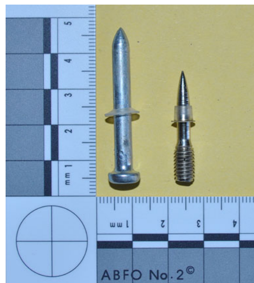
Fig. 6 Projectiles used for the test shots. Left , Drive pin (mass, m=6.825 g; maximum diameter, d=9 mm; length l=43 mm). Right , Threaded stud (mass, m=3.06 g; maximum diameter, d=6 mm; length l=30 mm). A plastic washer is mounted over the drive pin and stud to provide guidance and centring in the barrel
