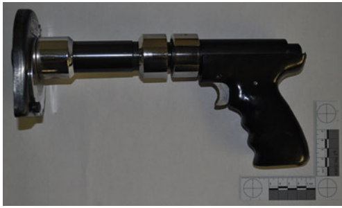
Fig. 3 Willi Kurschildgen “Titan Typ 1”; projectile diameter, d=6 mm, cartridge cal. 6.3/16 rimfire, proof test number PTB 61–69
