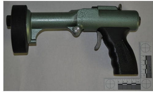
Fig. 5 Type “Ideal”; projectile diameter, d=9 mm, cartridge cal. 9×17 centerfire, no proof test number issued
