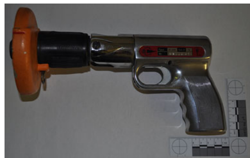
Fig. 2 Elektro-Feinmechanik Erich Holz “Rapid Hammer R300”, projectile diameter, d=6 mm; cartridge cal. 6.3/16 rimfire; proof test number PTB 63–69. Direct-acting power tools have to be equipped with a ricochet-preventing safety shield around the muzzle
